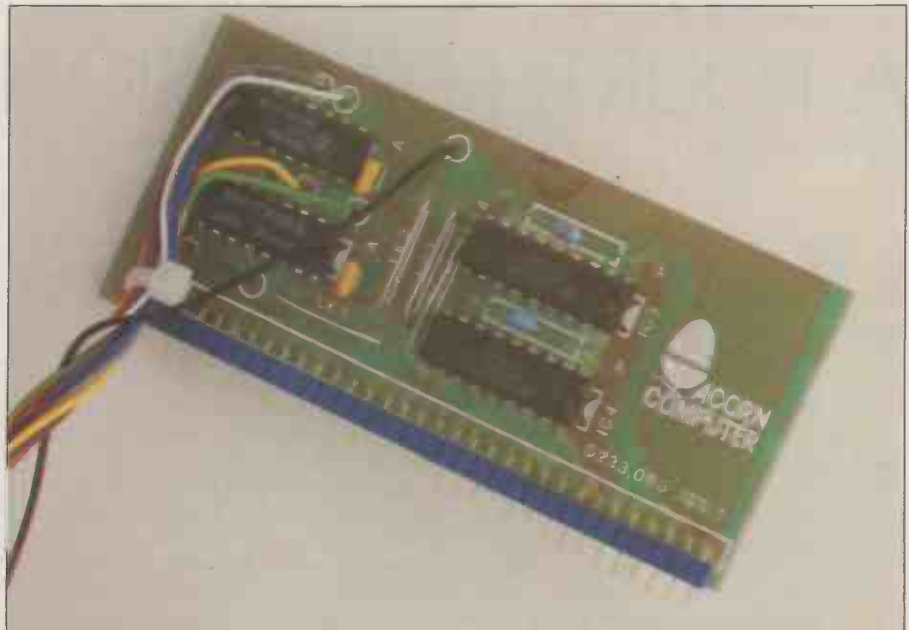
The daughter board adds 64K of RAM to the BBC B+, but it slugs the operating speed.
