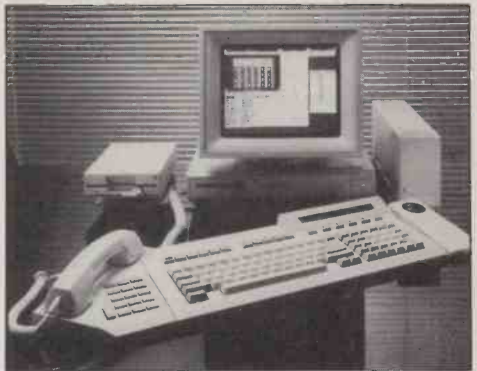
The Xen comes with an 80286 processor, MS-DOS and Windows.
